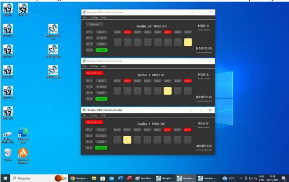
In the figure below, the RELEASE command was applied to Radio 1A. Note that only Radio 1A has disabled antennas.
