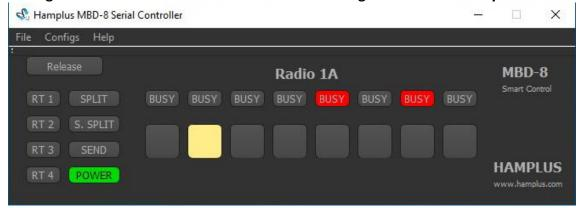
**The figure below** shows the **MBD-8** after activating the **RELEASE** command. Note that there is no activated antenna, only the **BUSY** indication on antennas 5 and 7 are being shown. This is because only this **MBD-8** released the antennas.
