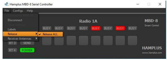
The figure below shows the RELEASE ALL Command activated (it is in red). When activated, all MBDs release their antennas.
