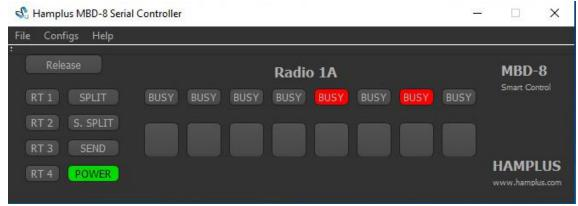
**The figure below** shows where to configure the **RELEASE** command to **release all MBDs** that are connected to the same **"BUSY"** network.
