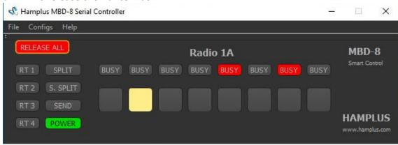
The figure below shows the MBD-8 after the RELEASE ALL command has been activated. Note that there is no indication of BUSY or Connected Antennas.
